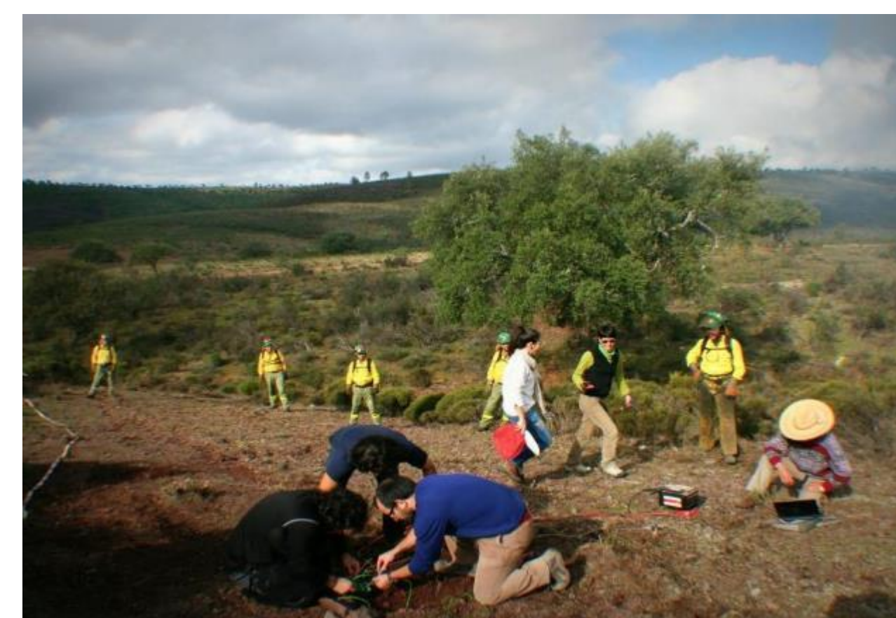
Figure 3. Installation of thermocouple probes.
