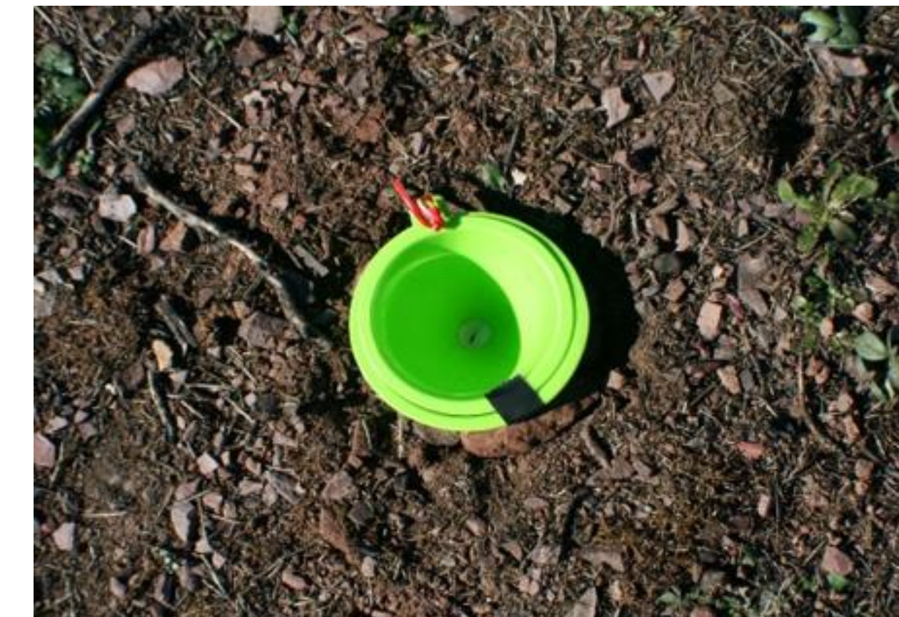
Figure 6. The sediment collector installed in the soil.
