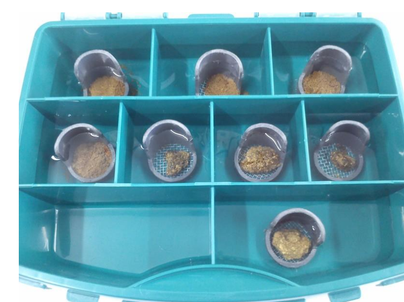
Figure 3. Detail of the stability to slaking test.
